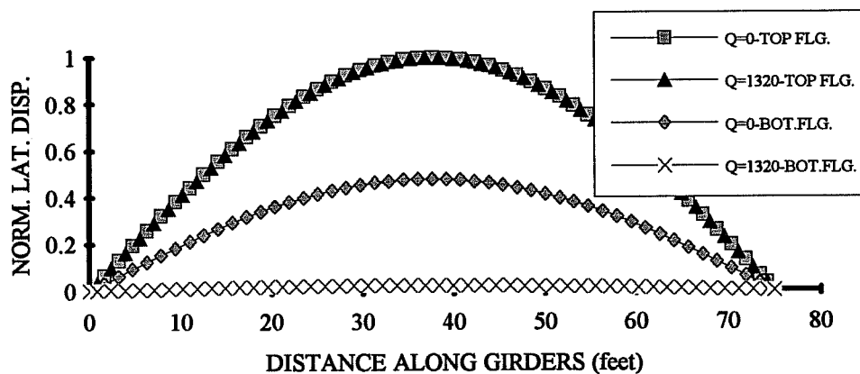
Figure 5.12b Lat. disp. of top and bot. flange for section #2, L = 75', Constant moment
